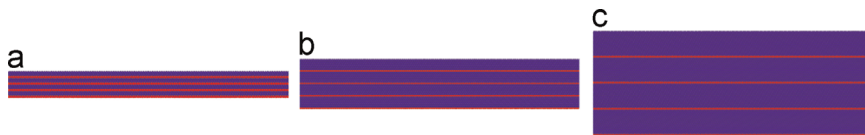
Fig. 7. Atomistic structure of a typical nanotwinned specimen with four CTB ( N=4 ) and different spacings d . The red atoms represent the CTBs: (a) d=0.6 nm, (b) d=1.8 nm, (c) d=3.0 nm. (For interpretation of the references to color in this figure caption, the reader is referred to the web version of this paper.)
