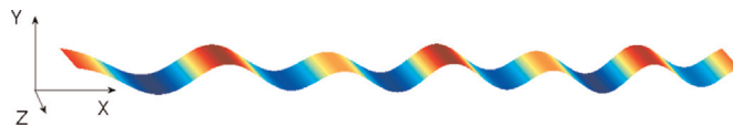
Fig. 3. A fluctuating membrane approximated as quasi-one-dimensional with b \ll W , where W is the length in the direction of wave propagation ( X -axis), and b is the width in the Z -direction. Different colors indicate different out of plane displacements. (For interpretation of the references to color in this figure caption, the reader is referred to the web version of this paper.)
